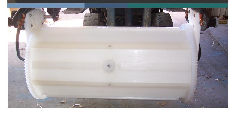
"Our door ribs are cut on an angle this gives the door a much tighter seal so parts don't get stuck in the door when plating."
